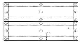
a = edge zone dimension = 10% of least horizontal dimension or 0.40h, whichever is smaller, but not less than either 4% of least dimension or 3 ft.
